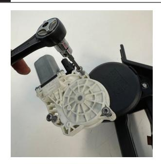
Secure the new gear cover onto the housing.
