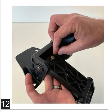
Insert the new motor into the housing. Using the supplied PT screws and a Torx T25 tool, tighten the screws. Torque to 36 in-lbs.
