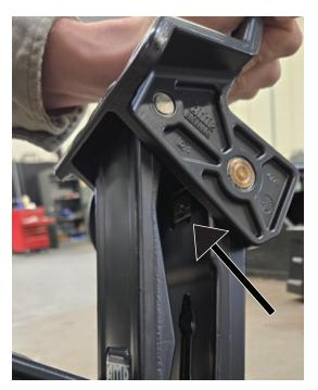
Remove the plastic gear cover from the housing.
