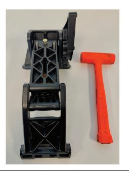
Pull drive shaft to remove from the linkage.
