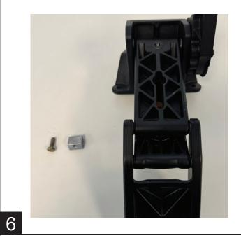
Using a 5mm Hex (Allen) key, remove the three bolts securing the gear housing to the linkage, and then remove the gear housing.
