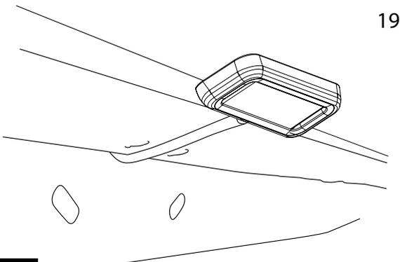
Using supplied butt connectors, connect the lamp wires. Red to Red, Black to Black
