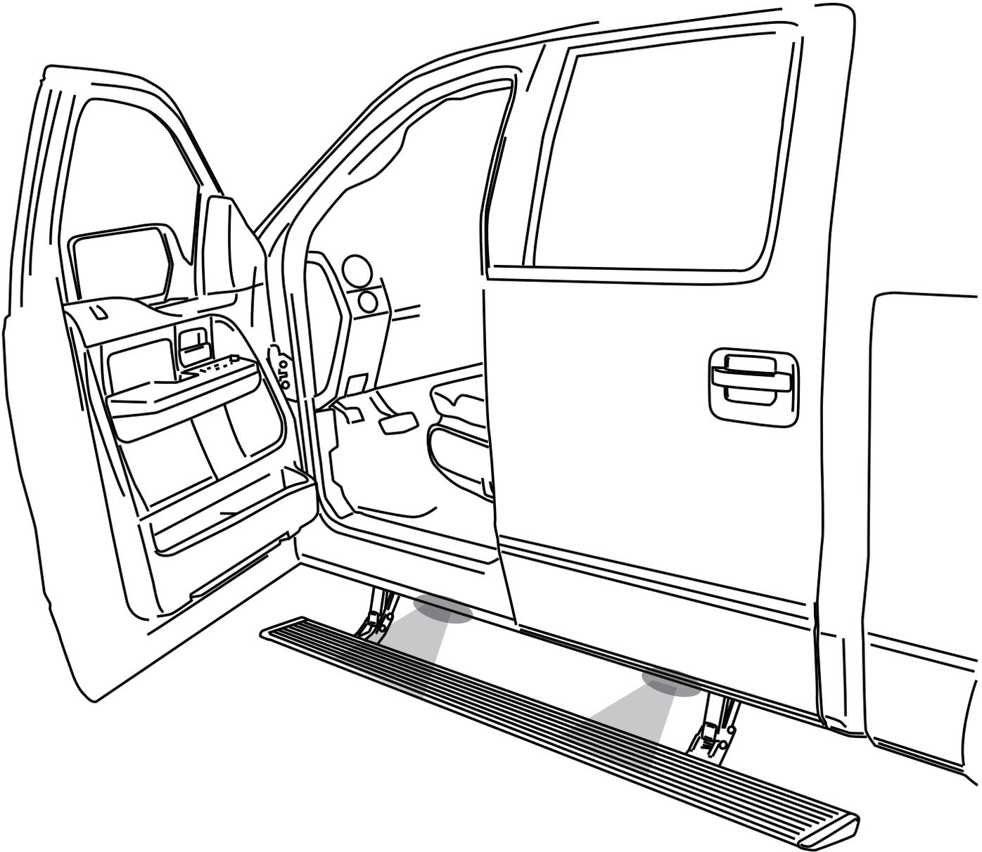
**Correct operation of Lights:** All four lamps will illuminate upon opening any door of vehicle. Lamps will stay on until restowing of both Power Steps or until 5 minutes has expired with the doors open. When the lights timeout after 5 minutes, they can be reilluminated by closing and opening any door of vehicle.
