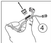
Connect red and black power leads to battery. Red lead goes to positive. Route shorter leg of harness down passenger-side wheel well.
