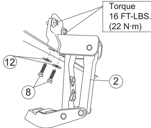
**Note:** Filing of sheet metal edge may be required if the sheet metal holes are misaligned.
