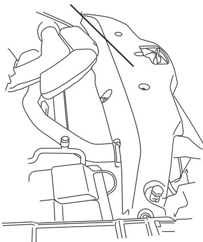
Mount controller with the two 11" tie wraps to factory conduit. Route wire harness under core support and down toward controller. Attach harness to controller (make sure connector locking tabs fully engage).
