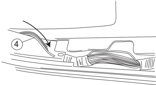
Locate the appropriate signal wires as noted below. Note: There may be up to five Black with Blue Stripe wires; use the one that looks unique (ie. different blue stripe... weight and shade).
