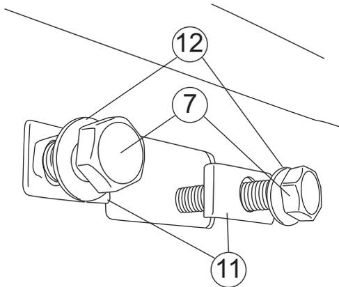
Mount idler assembly and motor assembly.
