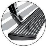
**POWERSTEP™ OPERATION** - The AMP Research PowerStep™ automatically deploys when any door is opened. When both front and rear doors are closed, it retracts automatically under your vehicle.
