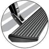
**POWERSTEP™ OPERATION** - The AMP Research PowerStep™ automatically deploys when any door is opened. When both front and rear doors are closed, it retracts automatically under your vehicle.
