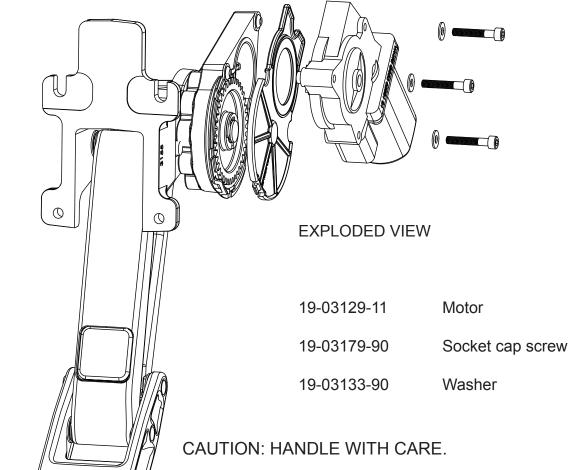
To insure our customers receive all components with full integrity, we pack the motors separate from their linkage assemblies. This requires that the installer position and fasten the motor before continuing with the install. Please follow the instructions below and handle the assembly carefully.
