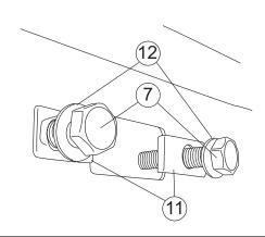
Mount idler assembly and motor assembly. Note: Filing of sheet metal edge may be required if the sheet metal holes are misaligned.
