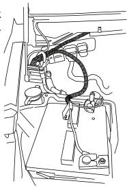
Route longer leg of harness down along driverside wheel well and along frame of vehicle. Secure with tie wraps.
