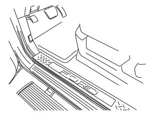
Remove tape from 3/4" hole in floor panel above front linkage on driver side and insert grommet. Thread the two trigger wires through grommet up into the cabin of vehicle. Seal grommet with silicone sealer.
