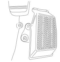
Pry up front door sill plates and remove kick panel fasteners and panels on driver and passenger side.
