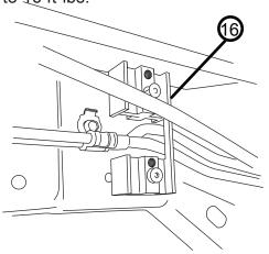
Pre thread upper M10 flange head bolt onto frame mount. Slide linkage into position and thread in lower flange head bolt. Motor faces
