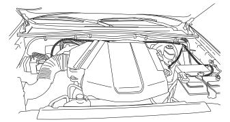
Note: Run loom with Green/Yellow and Pink/Black Trigger wires down drivers side of vehicle.
