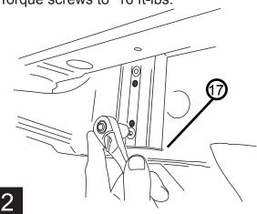
Pre thread upper M10 flange head bolt onto frame mount. Slide linkage into position and thread in lower flange head bolt.
