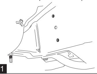
Using provided flat head cap screws attach frame mount extrusion to front set of threaded holes. Torque screws to 16 ft-lbs.
