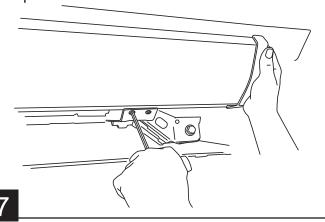
Attach motor onto Motor Linkage Assembly using two M6x16 flat head screws on both drive and passenger sides
