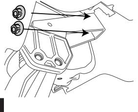
Insert threaded bracket into bumper and assemble bracket with supplied bolt. **Use slotted end of bracket at bolt.**
