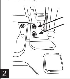
Install bracket to truck Torque nuts to 59 ft-lbs / 80Nm
