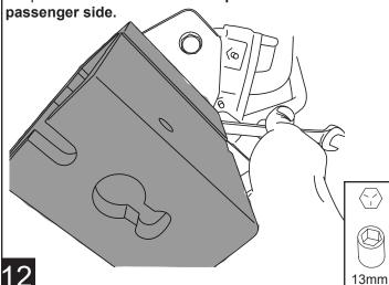
Set "Bracket E" and "Bracket D" together using provided flange head screw tighten bolts. Tighten bolts from Step 6 and 9. Torque to 16ft-lbs.
