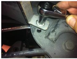
Note: Passenger side bracket will need supplied nut to tighten bracket into place. Use the upper hole. Do not tighten
