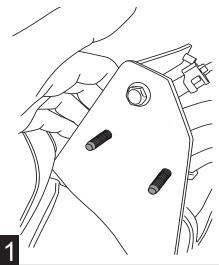
Set frame mount into position and tighten two bolts. Torque to 16 ft-lbs. **Note: See step 1 for orientation on passenger side.**
