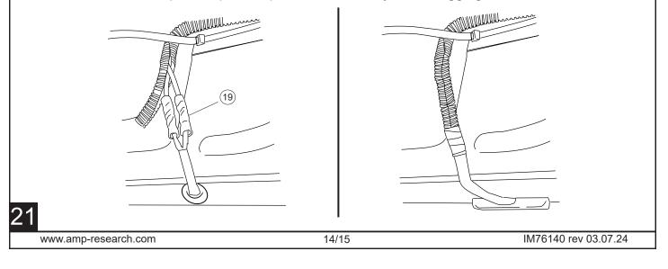
Insert plug from wire harness (4) onto motor (7). Slide rubber grommet on wire harness into slot of motor cover (8). Insert motor cover onto motor. Use electrical tape to cover any exposed wire from the motor. Insert plastic push pin rivets (14) in mounting holes of motor cover (8). Use pliers to ease installation. **NOTE: On 2 Door Bronco, tie up exra wires using supplied zip ties (15) to avoid wire snagging.**
