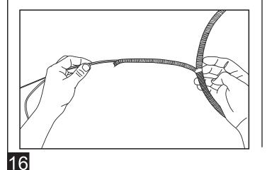
Locate oval grommet on driver side of firewall and push out. Poke small hole in grommet and thread trigger wires into cab of vehicle.
