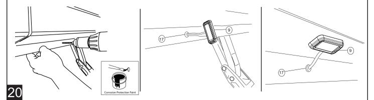
Using supplied butt connectors, connect the lamp wires. Red to Red, Black to Black. Once Crimped use heat gun to shrink tube. Close and wrap with conduit and electrical tape. Secure all loose wires with cable ties, with lamp wires pulled upward to avoid any wire snagging.
