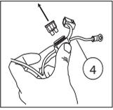
Attach wire harness to controller (make sure connector locking tabs fully engage). Mount controller with the two 11" tie wraps to factory conduit, just forward of battery.
