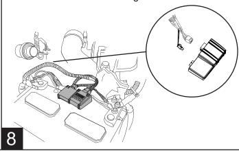
Connect power and ground for controller to battery, Red to positive and Black to the negative lead. Route harness legs down over wheel wells toward motor linkages, long leg across front and over to driver side. Secure all loose sections of the harness with cable ties.
