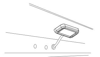
Using supplied butt connectors, connect the lamp wires. Red to Red, Black to Black. Once Crimped use heat gun to shrink tube.
