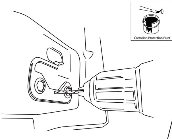
Once hole is drilled insert a piece of string or wire through hole in Reinforcement Plate(21). Set plate into position.
