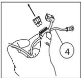
Connect red power lead to battery. Connect black ground lead to 13mm bolt outside of fender wall. Attach wire harness (4) to controller (5) (make sure the connector locking tabs fully engage). Mount controller with the two 11" tie wraps (16) to factory conduit, just forward of battery.
