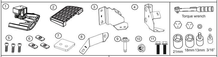
Assemble brackets as shown. **Spacer to be used on dual exhaust versions only!** 33 ft-lbs / 44 Nm
