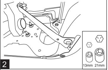
Remove 2 nuts and set assembly into position. Reuse factory nuts and Torque to 41ft-lbs/ 55N-m.
