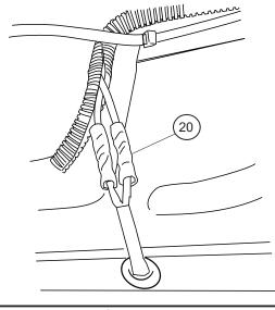
Drill a 9/32" hole through the pinch weld at marked locations. Debur all holes. After drilling apply paint to holes to provent rusting
