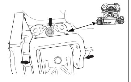
The jogs in the lower part of the linkages point toward one another, as shown, Drive (motor) Linkage in the Front and Idler Linkage in the Rear. Note: Linkage position described in parts list on page 3.
