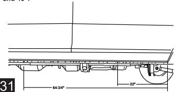
Insert grommet into drilled holes. Insert lamp wires through the grommets. (Silicon lube will help wires slip through grommets.)
