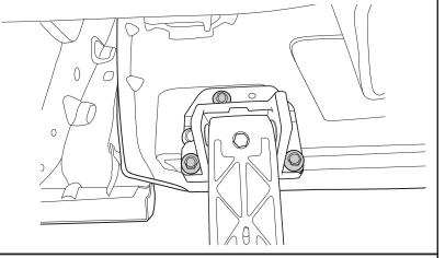
Set front body mount plate (26) to body. Driver side shown. Use supplied Conical washer bolts to attach as shown, At the pinch weld Use a T27 Torx driver and torque bolts to 6ft-lbs. Next torque bolts to 16 ft-lbs.
