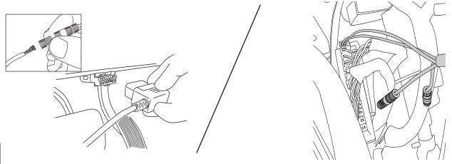
Secure harness with supplied tie wraps. Make sure wires are away from E-brake mechanism and brake pedal assembly.
