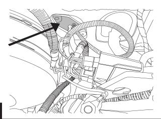
Tape leading end of wires together and push through rubber boot to cabin side of the firewall. Silicon lubricant may be used for ease of passage. The trigger wires will come out just above and to the left of the brake pedal.
