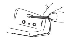
Rear Linkage Install: Set rear body mount plate (27) to body.
