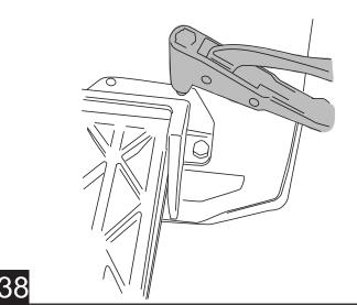
Reinstall fuse to Powerstep harness. Check that all doors activate the Power Step and the LED Lights work when doors open and close. Reinstall any remaining trim panels.
