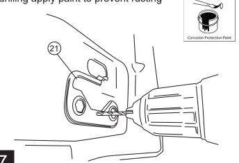
Once hole is drilled insert a piece of string or wire through hole in Reinforcement Plate. Set plate into position.
