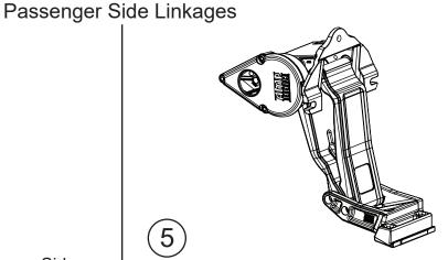
Motor Linkage Assembly - Passenger Side
