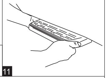
To deploy the step, press down using your foot on the outside edge of the step pad.
