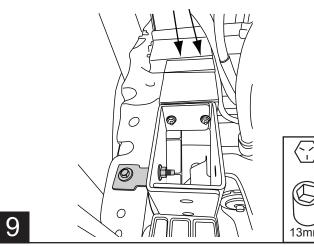
Verify step pad alignment to body line of vehicle.
