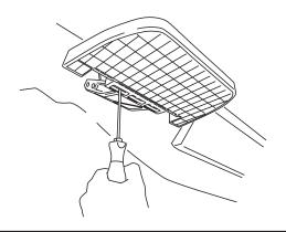
Using a 13mm Socket with extension. Torque to 16 Ft-lbs. Next torque bolts from step 8 to 16 Ft-lbs.
