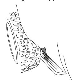
To retract, gently kick up on the underside of the step pad.
