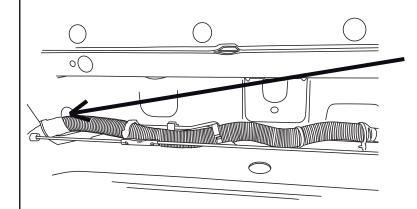
Route harness along the body mount bracket and zip tie to the factory harness. The purple wires will go through plastic plug in the floor in step 16.
