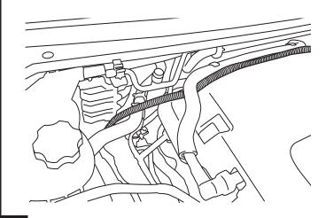
Route the passenger harness-leg down to the outside of the frame on the passenger side behind the inner fender liner, over the body mount bracket and to the motor on the front linkage. Secure with zip ties.
