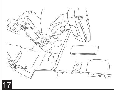
Lift the carpet to expose the plastic in-floor plug. Drill a 9/32" hole in the middle and insert the supplied rubber grommet (22).
