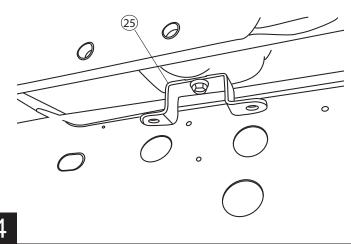
Snug the front linkage bracket (25) to the rivenut first. Note: bracket to be oriented closest to the frame.
