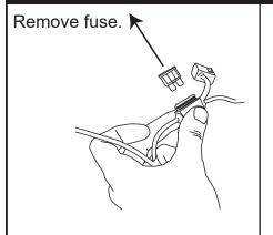
Remove Fuse from harness. Plug harness to controller and ensure that locking tabs are engaged. Attach controller horizontally to driver side wire loom. Secure with 11" cable ties. Attach ground lead to the negative battery terminal. Open the power distribution block cover and connect the Power wire to the positive power battery cable terminal.
