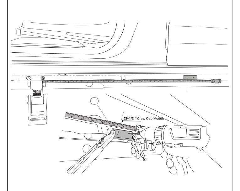
With drill template secured with vise grips, drill 1/8" Pilot holes. Remove template and drill holes to 21/64".
