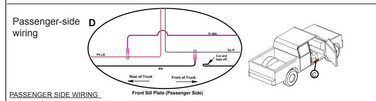
1. Remove passenger side front sill plate, open wire bundle and locate rear door-ajar wire (pink with light blue stripe). This wire will be located rear of junction where wires route under from passenger seat.
