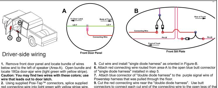
red connecting wire into light green with yellow stripe wire. 3. Route red wire into cab of vehicle and back toward sill plate area.
