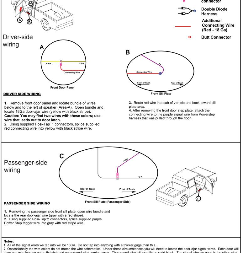
have one wire leading out to its latch and one ground wire coming away. The ground wire will usually be solid black. The signal wire we need is the other wire. 3. Make sure you secure all wires after install. Loose wires can be damaged and may cause a failure in the Powerstep's function.
