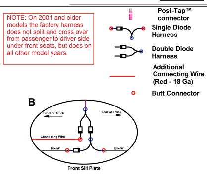
**4.** After removing the front sill plate, open wire bundle and locate rear door-ajar wire (black with a white stripe).
