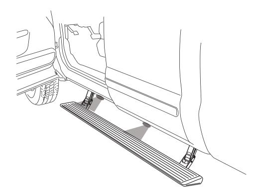
**Correct operation of Lights:** All four lamps will illuminate upon opening any door of vehicle. Lamps will stay on until restowing of both Power Steps or until 5 minutes has expired with the doors open. When the lights timeout after 5 minutes, they can be reilluminated by closing and opening any door of vehicle.
