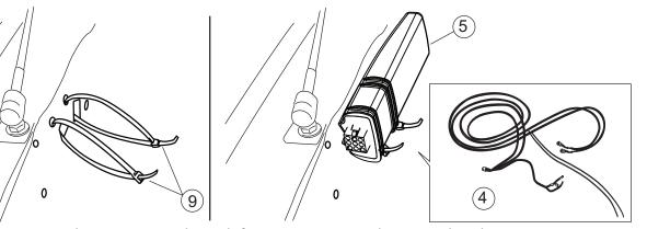
Loop two large tie wraps through fastener cutouts in sheet metal as shown. Position controller as shown above and cinch down tie wraps to secure controller in place. Connect harness to controller. Make sure that locking tabs on controller/harness connector are fully engaged.
