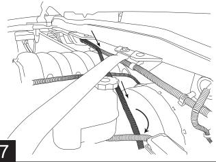
Pull up the carpet drill a 9/32" hole and thread both wires through the floor panel (add rubber grommet).
