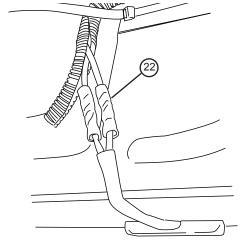
Close and wrap with conduit and electrical tape. Secure all loose wires with cable ties, with lamp wires pulled upward to avoid any wire snagging.
