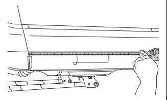
Affix lamp to rocker panel surface. Make sure the lamp is affixed to a clean, flat surface. There is a step down midway across the surface. Affix lamp just outside of step down.
