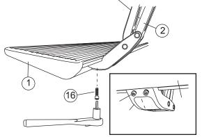
Tighten button head fasteners and M8 nuts on driving and idler linkages to 16 ft-lbs.
