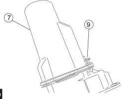
Slide motor assembly onto drive shaft and mounting bosses of driving linkage assembly. Use two (10) bolts to bolt motor down. Tighten to 16ft-lbs. Use electrical tape to cover any exposed wire from the motor.
